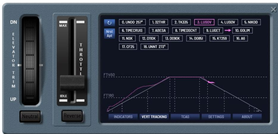
If the current flight plan is not displayed on the screen in the "**VERT TRACKING**" tab, or if there have been changes to the flight plan, click the "**Update**" button (with a round arrow).
