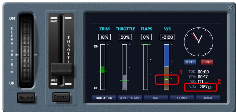
When the vertical speed indicator on the variometer is aligned with the marker (highlight **1** in the figure above), the aircraft will descend along the descent path of the active flight plan, as shown in the figure below.
